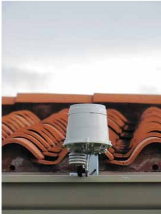
Figure 1. An example of an evapotranspiration sensor mounted on a roof. Credits: Michael Gutierrez, UF/IFAS
