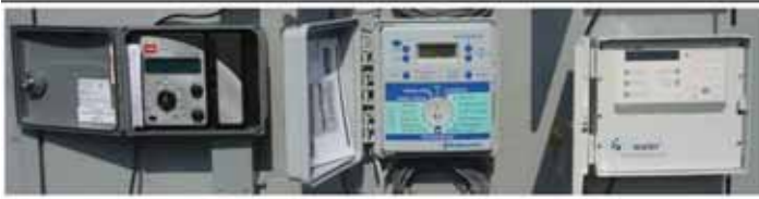
Figure 1. Photo of three brands of ET controllers undergoing testing at the University of Florida, Agricultural and Biological Engineering Department.
