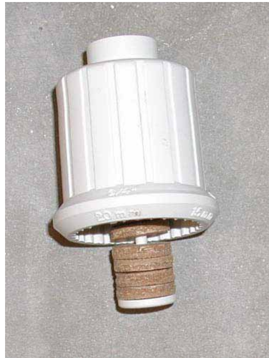
Figure 4. The expanding material of a shut-off device is visible in this photo of the cap removed from a device similar to the one in Figure 3.
