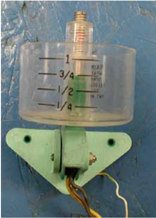
Figure 1. Weight-based rain shut-off device.
