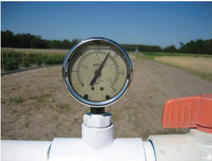
Figure 10. A fixed pressure gauge. Note the needle bathing in oil to prevent needle vibration and damage. Credits: Eric Simonne.
