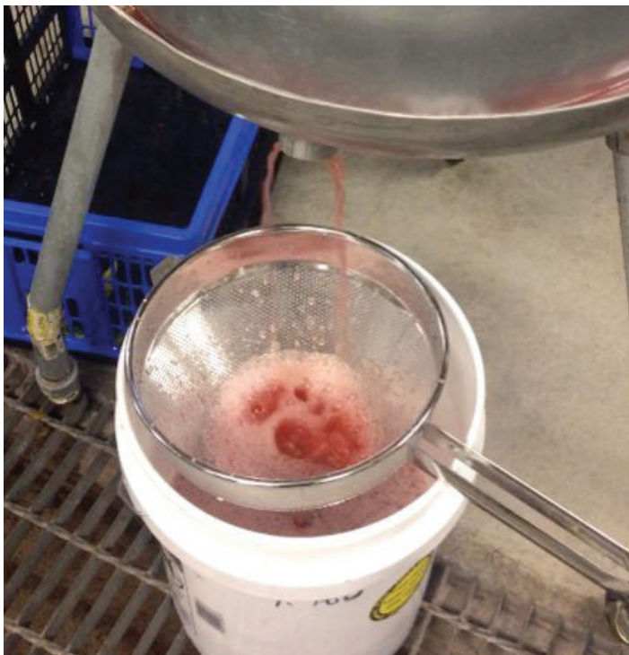
Figure 9. Using a colander to capture pulp and filter juice during peach pressing. Credits: Savanna J. Curtis, former graduate student, UF/IFAS
