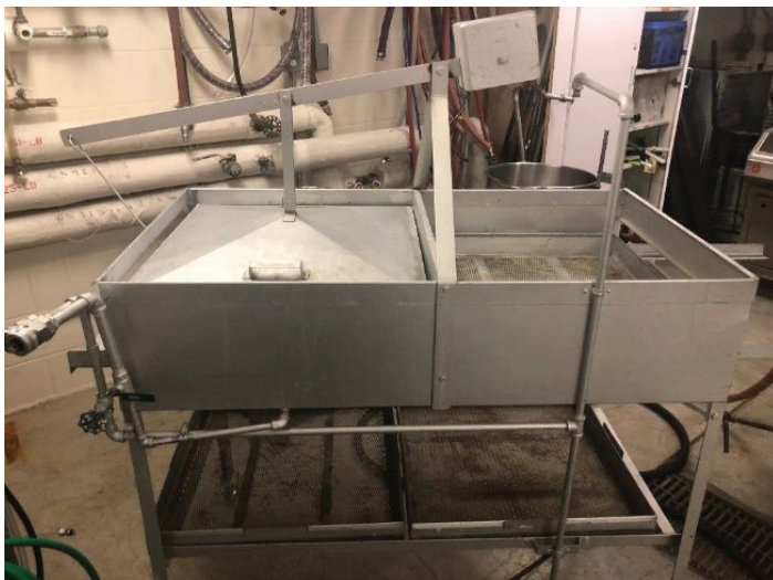
Figure 5. Steam blanching unit. Credits: Savanna J. Curtis, former graduate student, UF/IFAS
