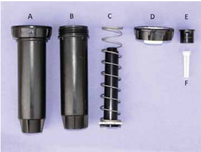
Figure 2. The components in a spray type sprinkler. The assembled spray is shown (A) along with the unassembled spray (B through F). The unassembled parts include the body (B), the spring and pop-up portion (C), the nozzle (E), and the filter (F). Credits: Bernard Cardenas-Lailhacar
