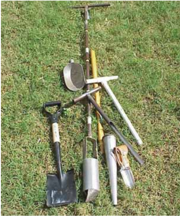
Figure 4. The collection of soil samples for nematode analysis can be acquired from the field using cylindrical sampling tubes, a trowel, a bucket auger, or a shovel.
