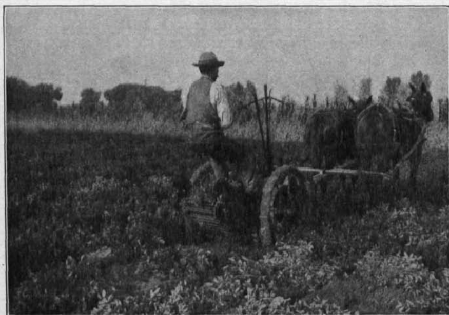
FIG. 9.—Machine potato digger in use in digging peanuts.
