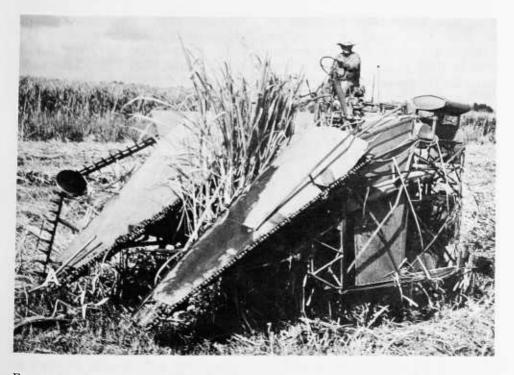
FIGURE 28. – Sugarcane harvester, illustrating pickup attachment (A) for harvesting lodged sugarcane.
