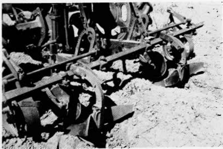
FIGURE 11.—Two-row lister used for plowing out middle area between beds after sugarcane is planted.
