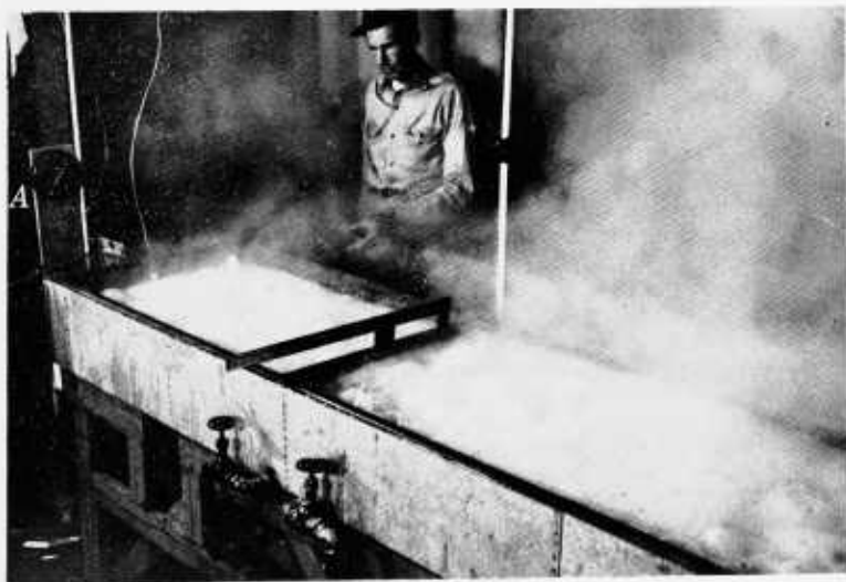
FIGURE 20.—Stubbs-type evaporator in operation. Thermometer ( A ) used to determine sirup density.
